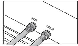
7. Turn on the HOT and COLD water supplies and check all the water supply intake connections and the faucets for water leaks.
