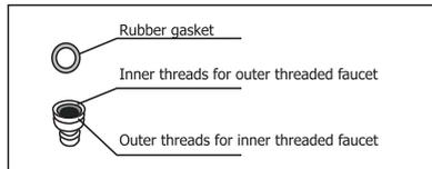
2. Connect the ends of the water supply hoses to the HOT and COLD faucets. For convenience, use the Quick Connection Adaptor for connection to the cold water faucet. See instructions for Quick Connection Adaptor use in Step 1 above.
